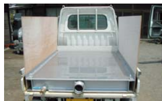
Small truck steam chamber 1.5m 3
